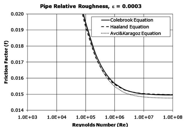
Fig. 1 Comparison of Eqs. (1), (3), and (4) for low pipe relative roughness
