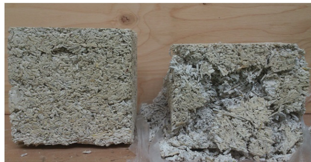
FIGURE 7. The form of destruction of an exemplary composite sample after a compression test
