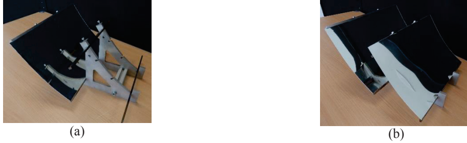
FIGURE 6. Prototype version V1. (a) View of the mirror M1 mounted and bare parabolic rib support prior to mounting mirror M2. (b) Full mounted V1 prototype.
