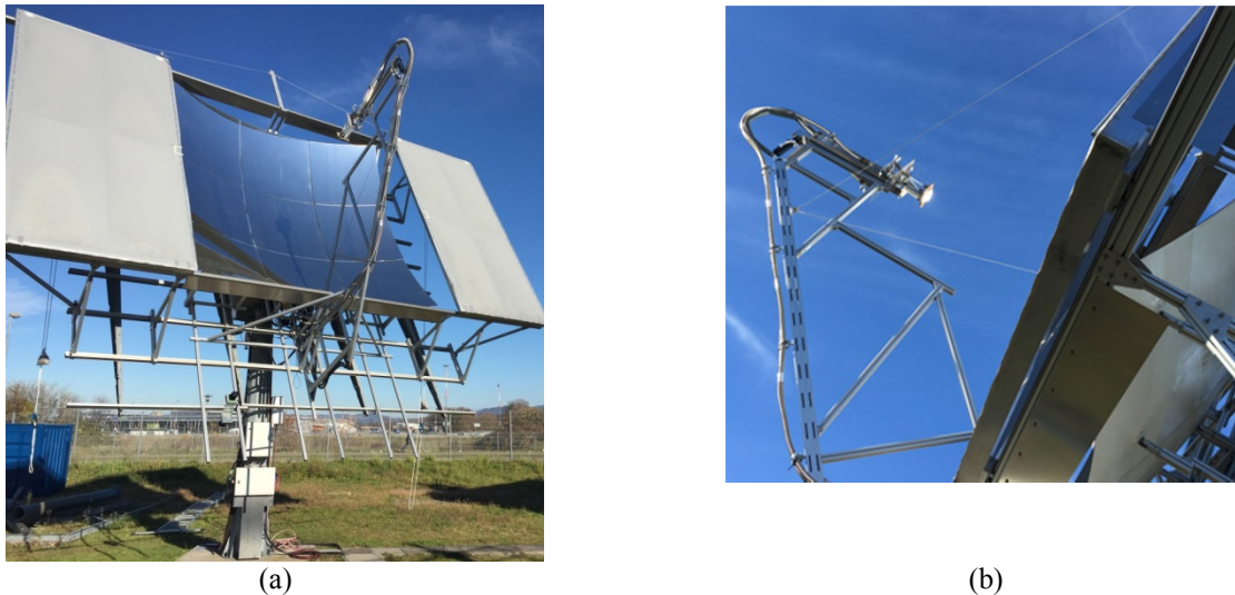
FIGURE 2. CPV dish system in Freiburg during start-up of the system on 10/11/2015. Left: complete CPV system. Right: illuminated thermal receiver.
