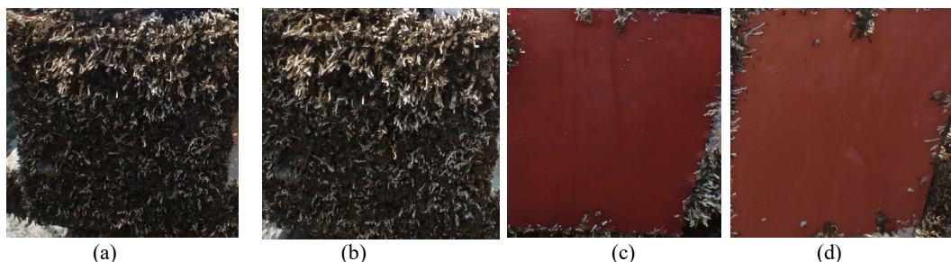
FIGURE 1. Biofouling formation on panels coated with anticorrosion A (a), antifouling A (b), anticorrosion B (c) and antifouling B (d) paints after 1 month of immersion in seawater of Jakarta Bay (The data from the same research has been reported [9])
