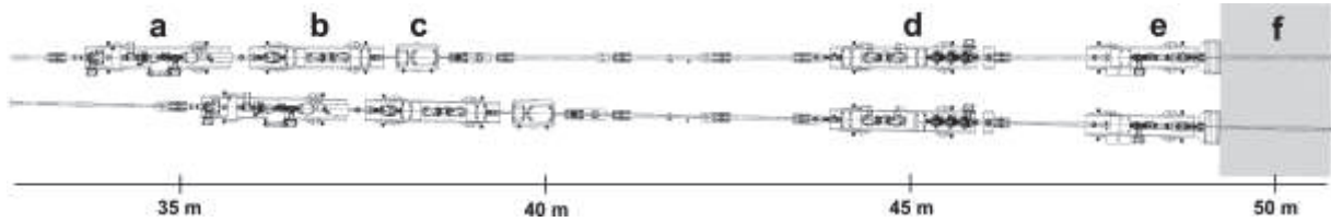
FIGURE 3 Frontend of a canted undulator sector. a: CVD diamond screen and vacuum valve b: vertical slits c: dump magnet d: vert./hor. photon shutter slit system and filter unit e: Bremsstrahlung collimator and beamstop f: concrete shielding wall
