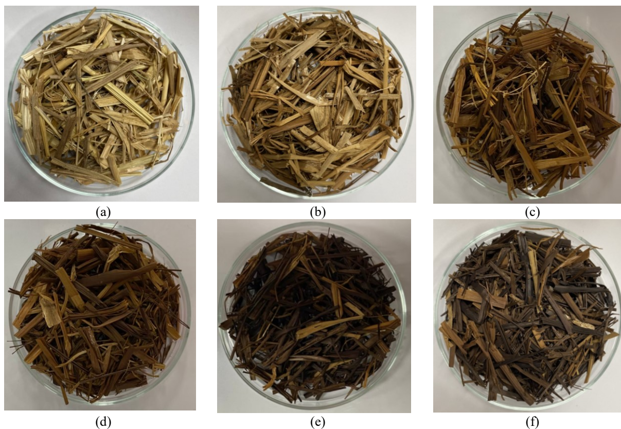
FIGURE 2. (a) Raw rice straw, (b) Torrefied rice straw at 200°C and 40 min, (c) Torrefied rice straw at 215°C and 30 min, (d) Torrefied rice straw at 215°C and 50 min, (e) Torrefied rice straw at 250°C and 25.7 min and (f) Torrefied rice straw at 250°C and 40 min
