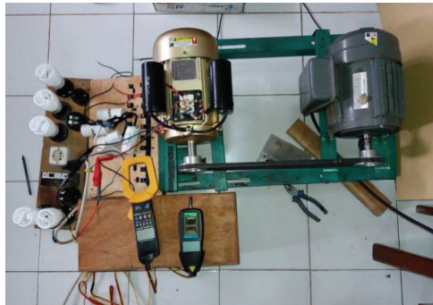
FIGURE 1. The experiment set-up to test the single-phase induction generator
