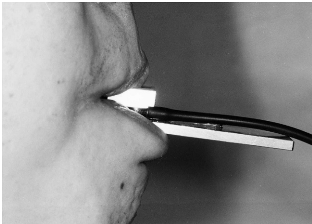
Figure 5. Lip closing force measurement using Y-meter.
