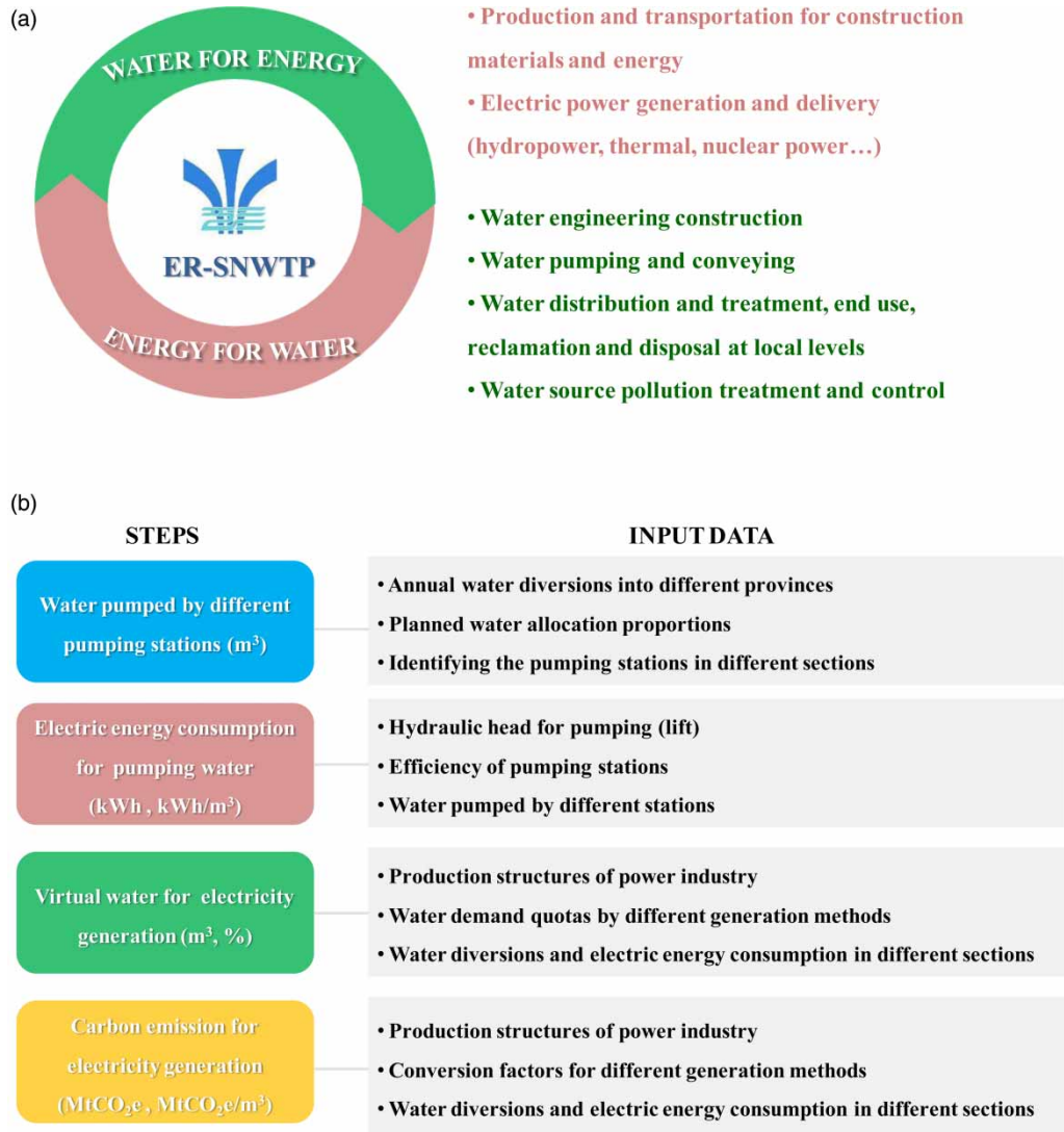
Fig. 2. A conceptual framework for water–energy nexus of the Eastern Route. (a) Linkage between water and energy in the Eastern Route; (b) methodological steps and data input for the estimations.
