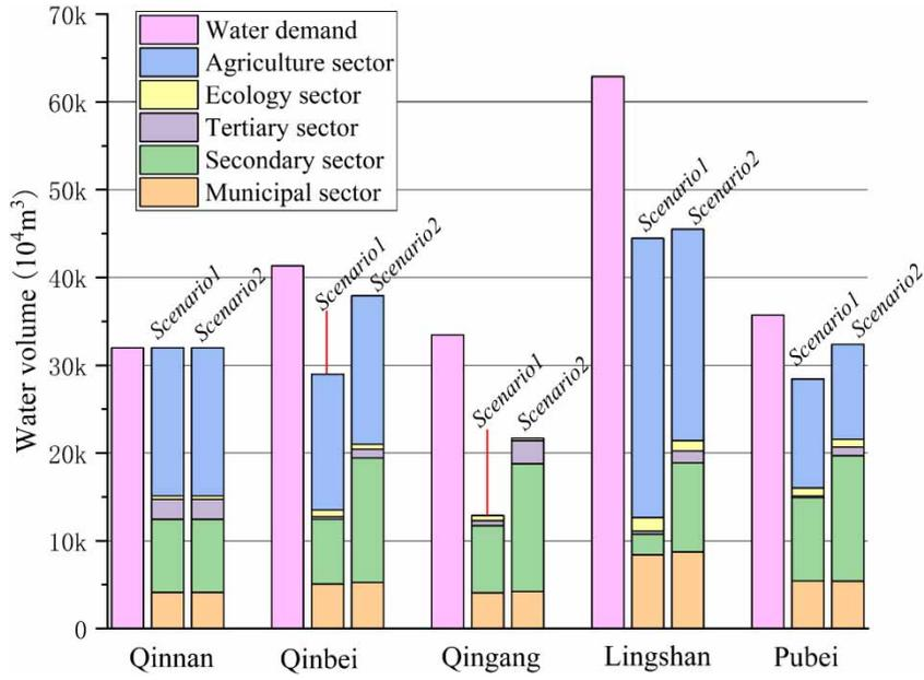
Fig. 4. Water volume allocation results for 2030.
