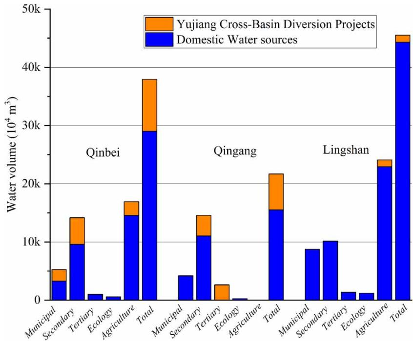
Fig. 5. Water volume allocation from Yujiang CBDP.
