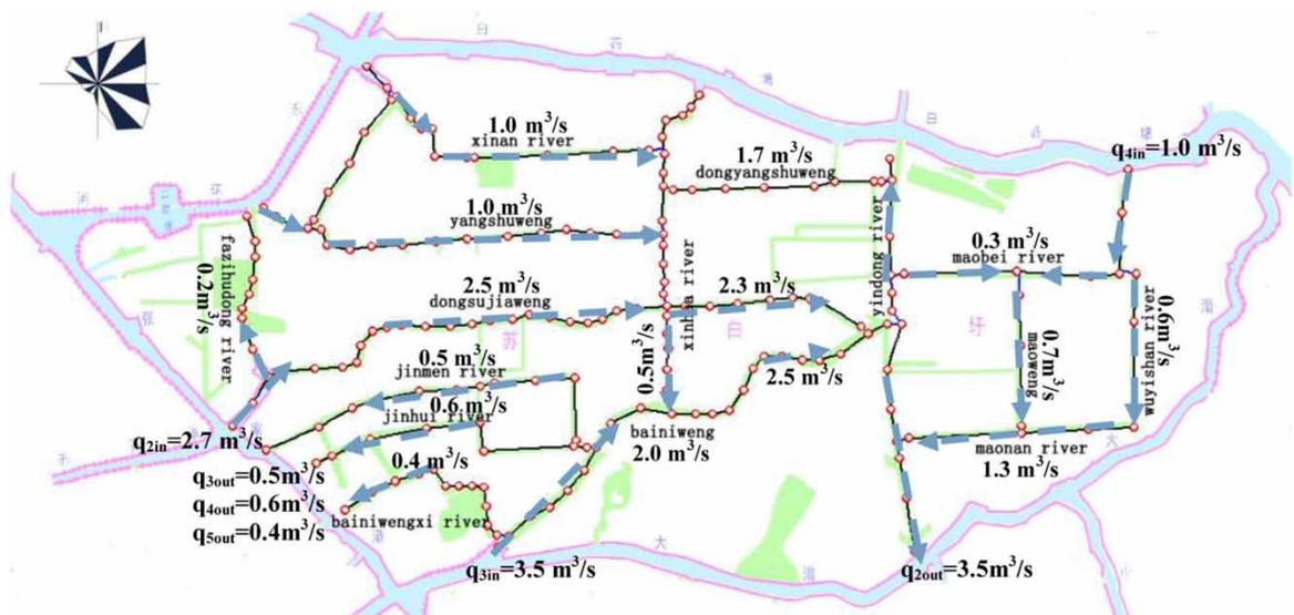
Fig. 5. Flow distribution of main node in the final scheme.
