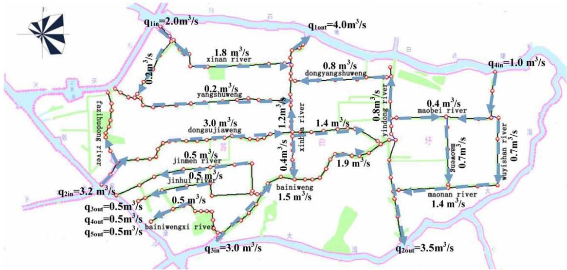
Fig. 3. Flow distribution of main node in preliminary scheme.
