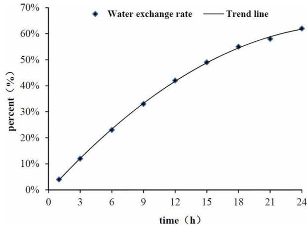
Fig. 6. The relationship curve between average water exchange rates and water diversion durations under optimized pumping scheme.
