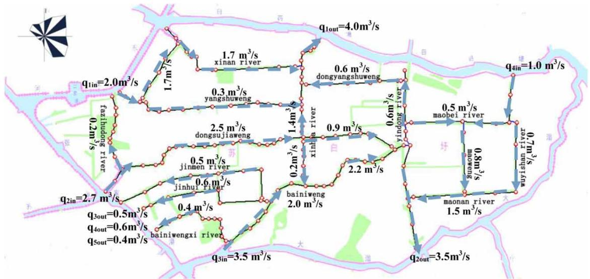
Fig. 4. Flow distribution of main node in optimized scheme.
