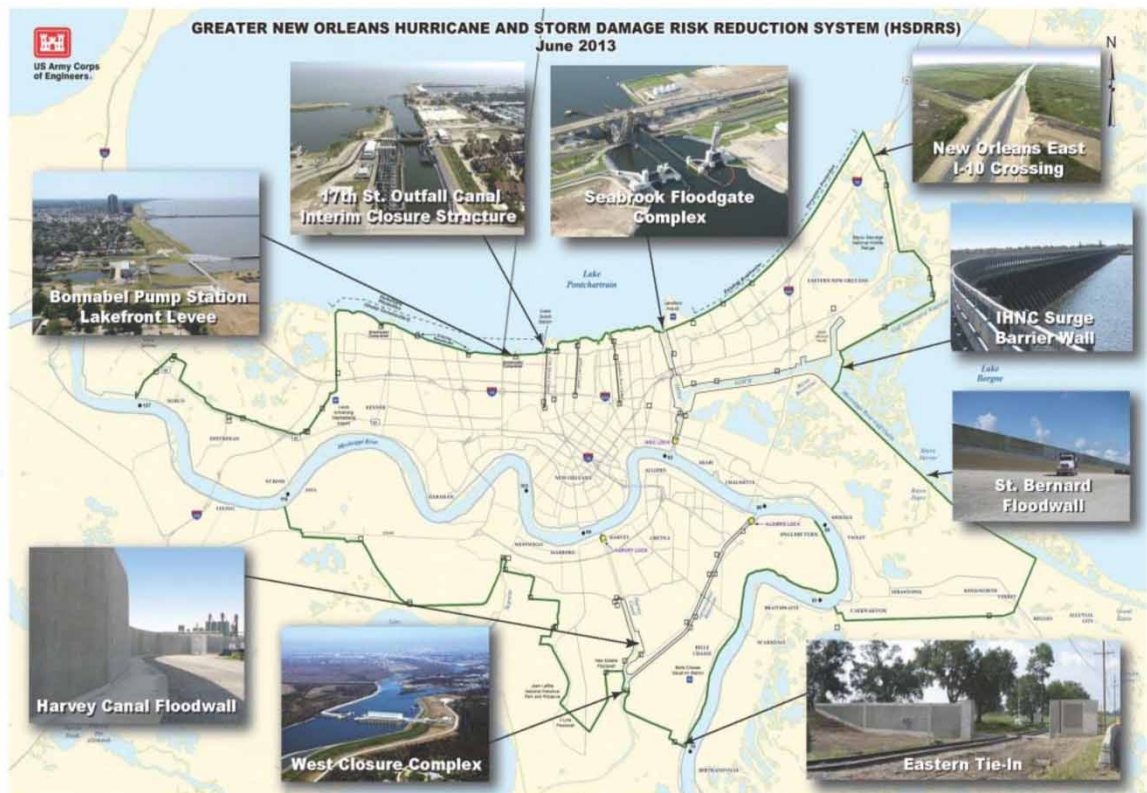
Fig. 1 | Map of the HSDRRS depicting the major structural components that were constructed in addition to broad increases in flood wall and levee elevation and strength, June 2013 (Source: Corps of Engineers).
