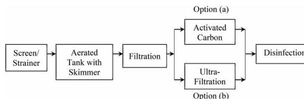
Fig. 6. Current GW treatment systems in Sharjah: (a) activated carbon; (b) ultra-filtration.
