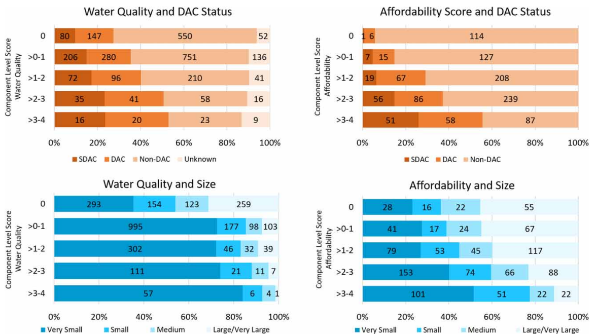
Fig. 4 | Bar charts indicating larger proportions of water systems serving disadvantaged and smaller systems have higher scores (i.e., worse outcomes/greater challenges) for water quality and affordability. Disadvantaged status defined using state definitions for DACs and SDACs, as those whose Median Household Income (MHI) is below 80 or 60% of statewide MHI. System size is measured by the number of service connections, with the following cutoffs: very small (1–200), small (201–999), medium (1,000–3,000) and large/very large (>3,300). Percent of systems on x-axis, number of systems indicated within each bar. N = 2,839 for water quality (i.e., 100% coverage) and n = 1,141 for affordability.
