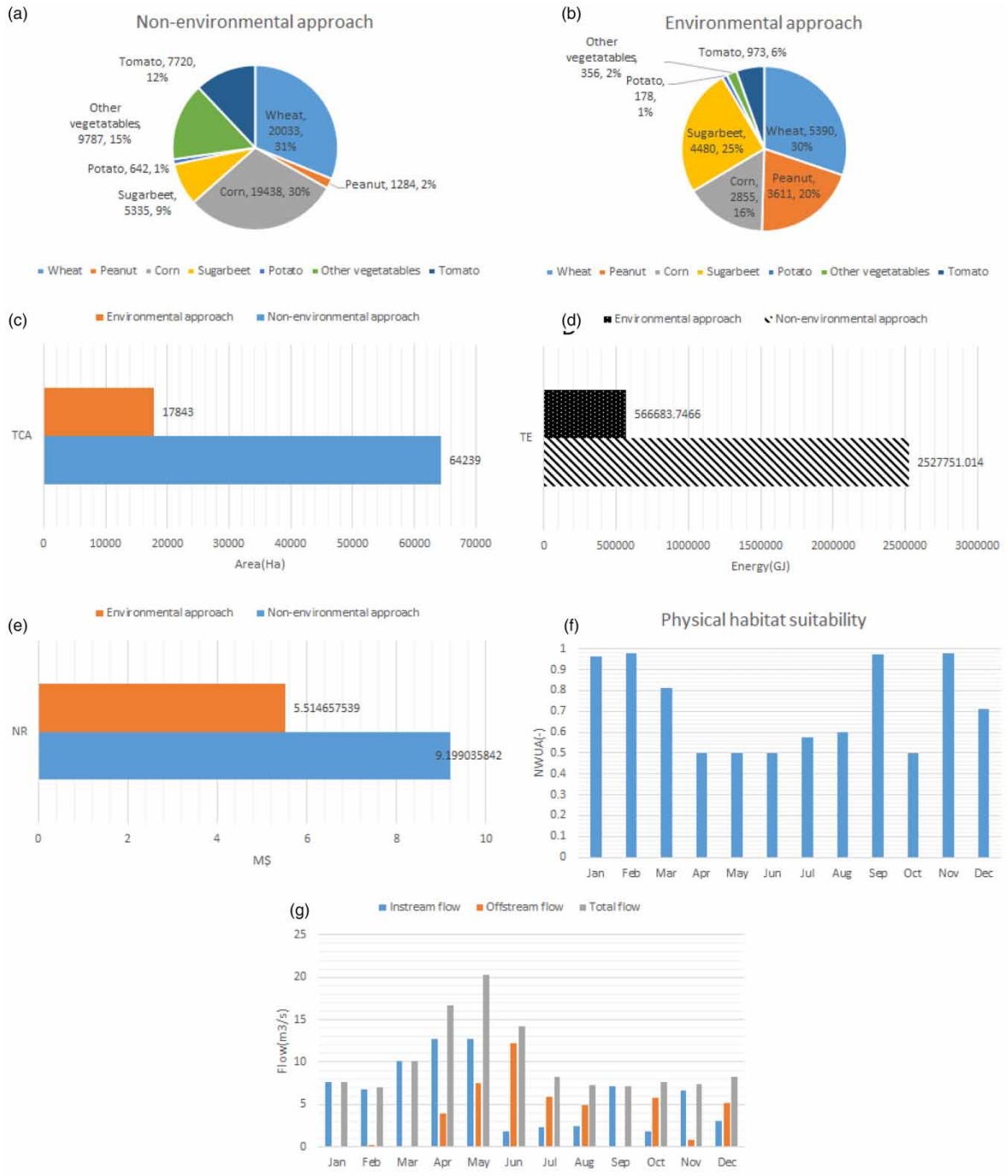
Fig. 6 | Output of the optimization systems in dry years (a: cropping pattern by the non-environmental approach, b: cropping pattern by the environmental approach, c: total cultivated area in each approach, d: total energy use in each approach, e: net revenue converted to M$, f: physical habitat suitability time series proposed by the environmental approach and g: proposed environmental flow (instream flow) and total and offstream flow by the optimization model).
