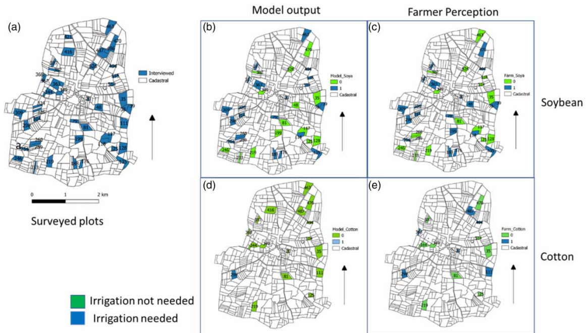
Fig. 9 | Kharif dry spell vulnerability in 2021 monsoon for Adgaon (a) interviewed farm plots, (b and d) dry spell sensitivity map in terms of irrigation requirement for (b) soybean and (d) cotton based on farmers' soil descriptions (assumes irrigation not needed when crop water deficit is \leq 15 mm, and irrigation needed when deficit is more than 15 mm), (c and e) farmers' descriptions of whether irrigation was needed in 2021 monsoon for (c) soybean and (e) cotton. (0 = no need; 1 = needed). Cadastral map sourced from the government of Maharashtra Maha-bhulekh.
