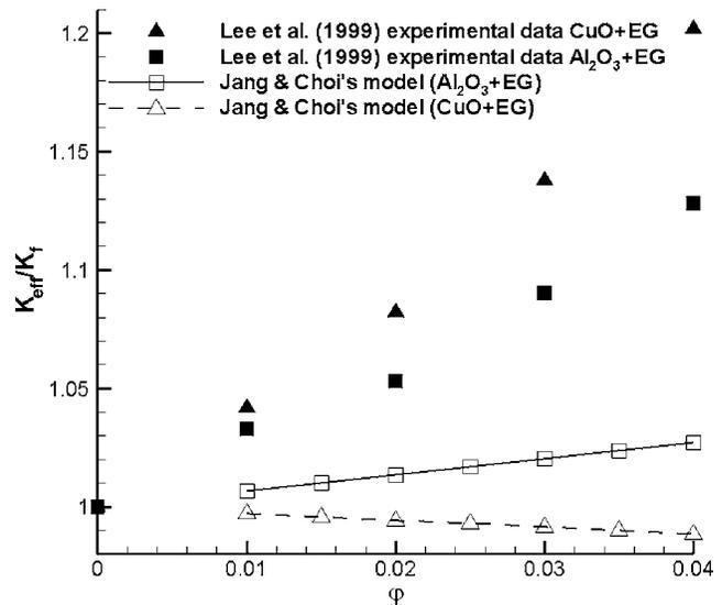
Fig. 3 Comparison of the experimental data (Lee et al. [12]) for Al<sub>2</sub>O<sub>3</sub>-EG and CuO-EG nanofluids with Jang and Choi's [3] model
