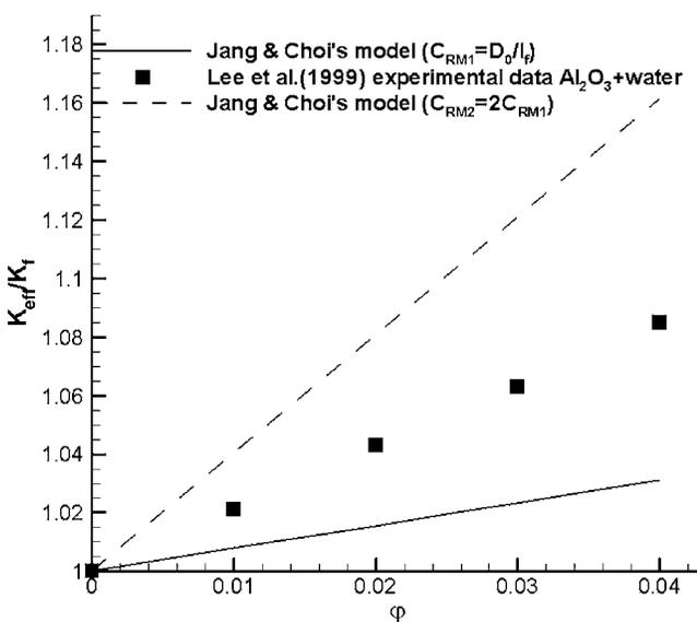
Fig. 2 Comparison of the experimental data (Lee et al. [12]) for Al<sub>2</sub>O<sub>3</sub>-water nanofluids with Jang and Choi's [3] model for different random motion velocity definitions
