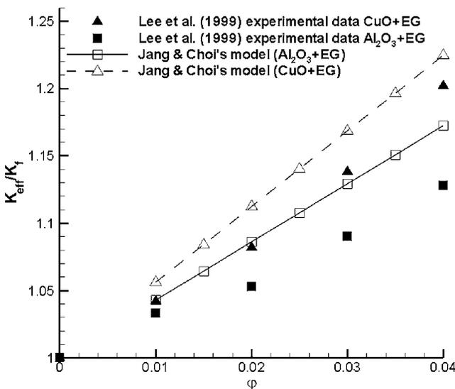
Fig. 6 Comparison of the experimental data (Lee et al. [12]) for  $\text{Al}_2\text{O}_3$ -EG and CuO-EG nanofluids with Jang and Choi's [3] model (new proportionality constant and new particle diameters are applied)
