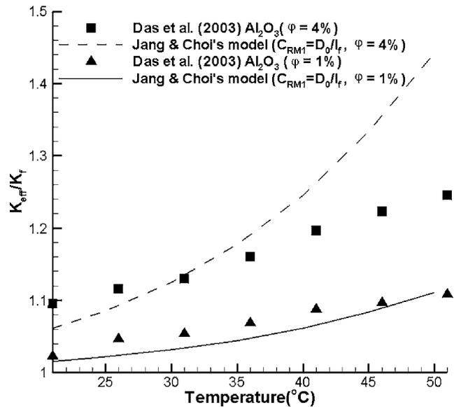
Fig. 7 Comparison of the experimental data (Das et al. [16]) for 1% and 4%  $\text{Al}_2\text{O}_3$ -water nanofluids with Jang and Choi's [3] model (new proportionality constant and new particle diameters are applied)
