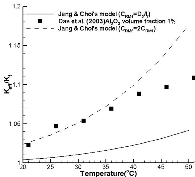
Fig. 4 Comparison of the experimental data (Das et al. [16]) for 1% Al<sub>2</sub>O<sub>3</sub>-water nanofluids with Jang and Choi's [3] model for different random motion velocity definitions
