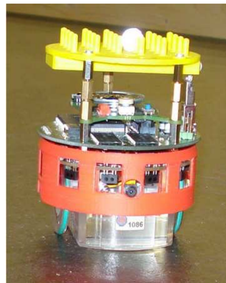
Figure 1: A Linux-extended e-puck robot. The robots are fitted with coloured skirts, to enable them to ‘see’ each other. The yellow hat on top of the robot provides a matrix of pins holding unique patterns of reflective markers that allow the tracking system to identify and track each robot.
