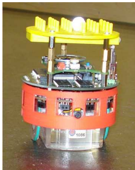
Figure 1: A Linux-extended e-puck robot. The robots are fitted with coloured skirts, to enable them to ‘see’ each other. The yellow hat on top of the robot provides a matrix of pins holding unique patterns of reflective markers that allow the tracking system to identify and track each robot.
