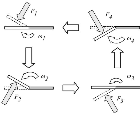
Figure 16: Mechanism generating propulsion
