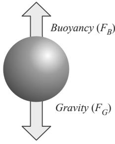
Figure 1: Modeling buoyancy
