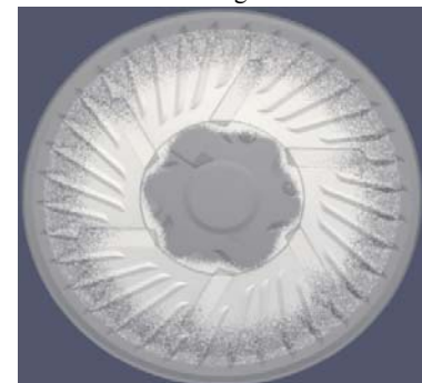
FIGURE 5. Particle distribution after 7 seconds process time (5040 angle steps)
