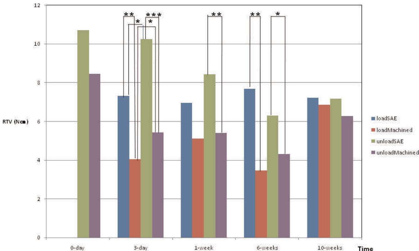
**Figure 5.** Removal torque value measurements after different loading periods between SAE and machined mini-implants. Statistical analyses are shown on the graphs. \* $P < .05$ ; \*\* $P < .01$ ; \*\*\* $P < .001$ .
