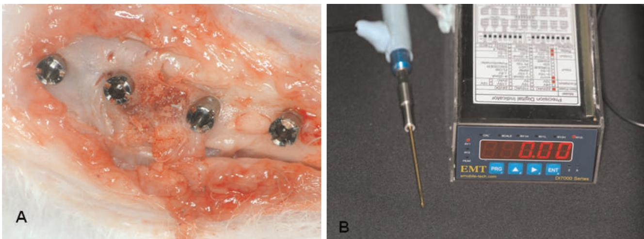
**Figure 3.** (A) The screw parts placed in the rabbit tibia before removal. (B) Torque driver with digital torque sensor with 0.01-Ncm accuracy.
