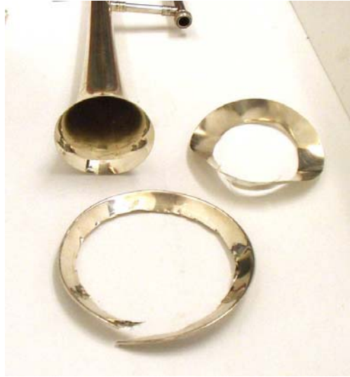
FIGURE 1: Boosey and Hawkes medium bored trombone (AM1229), showing fully cut state with two previously removed annular bell sections.
