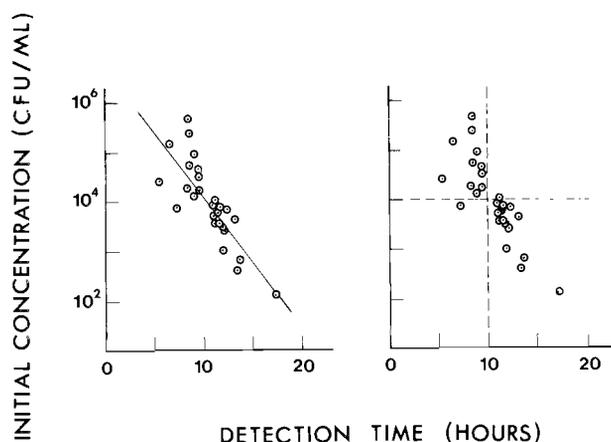
Figure 6. Scattergram of impedance response detection times (averages of duplicate channels) for 27 raw milk samples graphed against initial microorganism concentration as determined by plate count at 32 C. The solid line on the left side is the least squares linear fit to the data. The broken lines on the right side illustrate a scheme by which samples could be classified as having more than or less than  $10^4$  organisms/ml.
