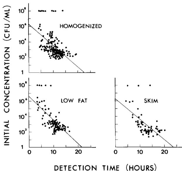
Figure 7. Scattergrams of impedance response detection times (averages of duplicate channels) graphed against initial microorganism concentration as determined by plate count at 32 C for 191 homogenized, 119 low fat, and 70 skim milk samples. The solid lines are the least squares linear fits to the data.
