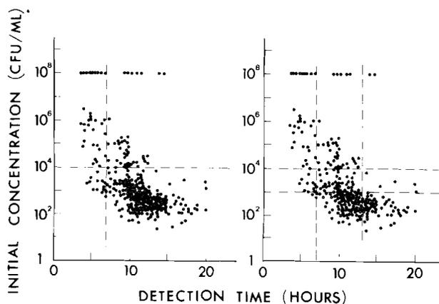
Figure 8. Scattergram of impedance response detection times (averages of duplicate channels) graphed against initial microorganism concentration as determined by plate count at 32 C for 380 samples of pasteurized milk. The dashed lines indicate two-way (left side) and three-way (right side) classification schemes applied to these data.
