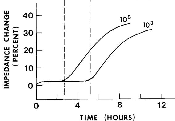
Figure 4. Relationship between microorganism growth (top) and impedance response (bottom) which makes possible the method of estimating initial microorganism concentration from impedance response detection times.
