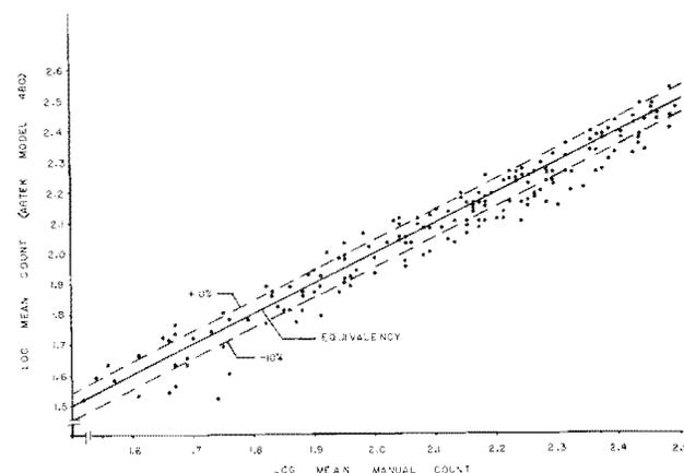
Figure 2. Scatter plot relating plate counts determined by Artek 480 to manual technique. Linear regression equation:  $Artek\ 480\ counts = 0.148 + (0.924 \times manual\ count)$ .
