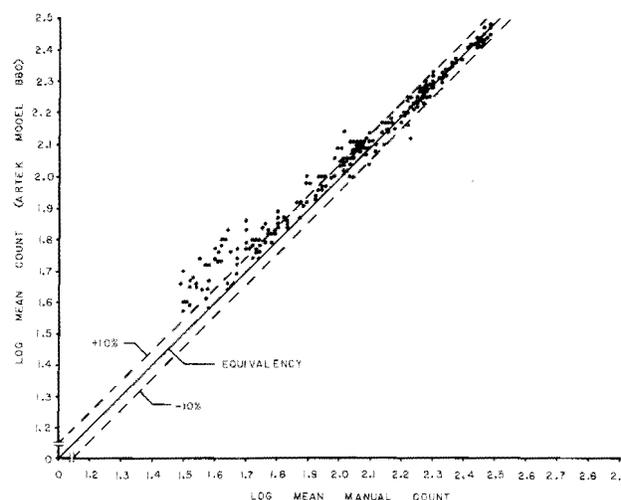
Figure 4. Scatter plot relating plate counts determined by Artek 880 to manual technique. Linear regression equation: Artek 880 count = 0.304 + (0.866 × manual count).
