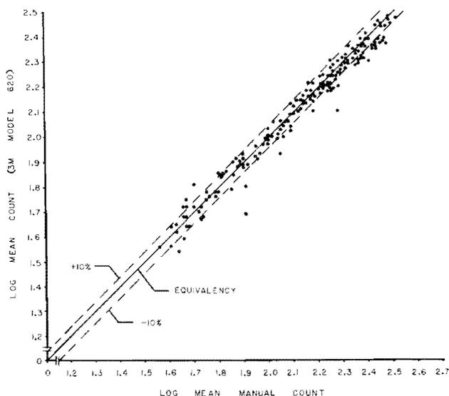
Figure 1. Scatter plot relating plate counts determined by 3M 620 to manual technique. Linear regression equation:  $3M\ 620\ count = 0.069 + (0.960 \times manual\ count)$ .
