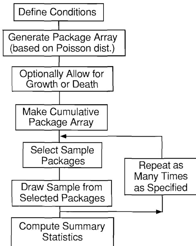
Figure 1. Flow diagram of computer program which performs simulation of package sampling and microbiological examination.
