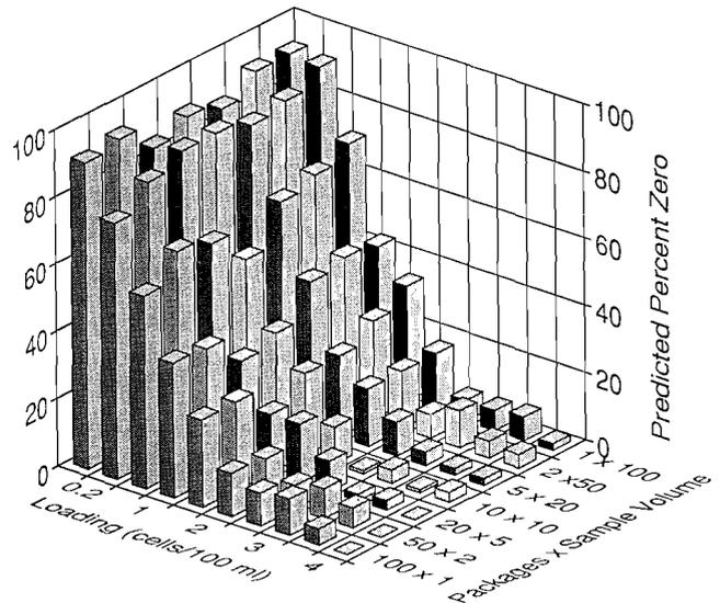
Figure 11. Predicted frequency of finding no counts in any sample in 100 simulations in which a total of 100 ml was taken from 1, 2, 5, 10, 20, 50, or 100 packages.
