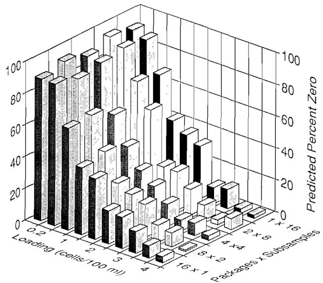
Figure 10. Predicted frequency of finding no counts in any sample in 100 simulations in which 16 total samples of 5 ml were taken from 1, 2, 4, 8, or 16 packages for each indicated organism concentration.
