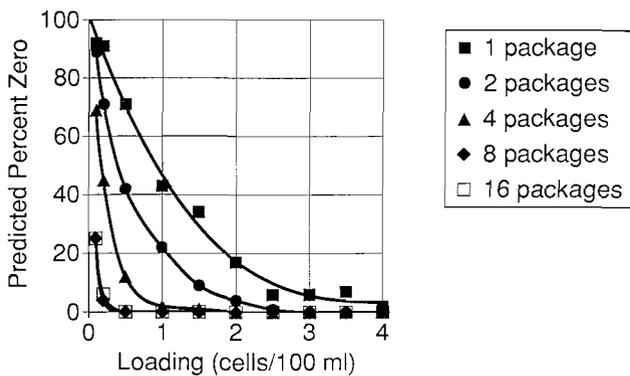
Figure 9. Predicted frequency of finding no counts in any sample in 100 simulations in which one 100-ml sample was taken from each of the number of packages indicated in the legend for each indicated organism concentration.
