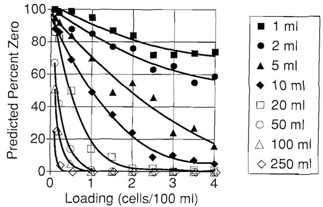
Figure 6. Predicted frequency of finding no counts in any sample in 100 simulations where the volumes indicated in the legend were withdrawn from each of 8 packages at each indicated organism concentration.
