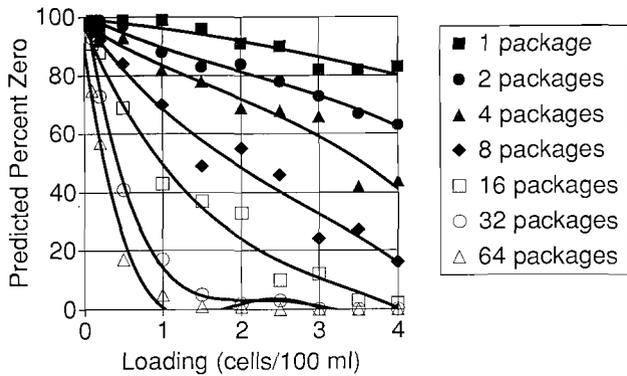
Figure 8. Predicted frequency of finding no counts in any sample in 100 simulations in which one 5-ml sample was taken from each of the number of packages indicated in the legend for each indicated organism concentration.
