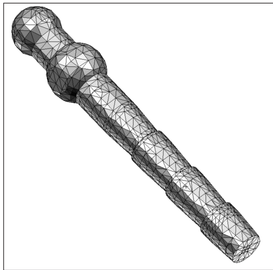
Figure 3: Mesh considered for the post.
