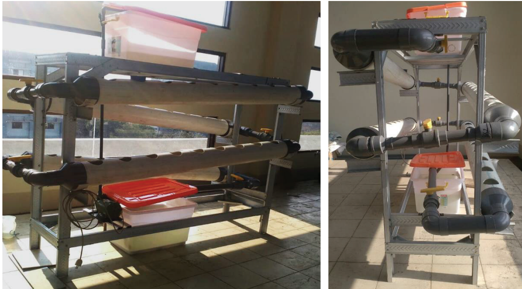
FIGURE 2. Final construction of the hydroponic system. There is a valve addition at the end of the fourth main pipe
