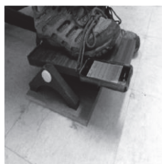
FIGURE 1. Ankle rehabilitation system with subject’s foot mounted to footplate and smartphone wireless gyroscope platform [8]
