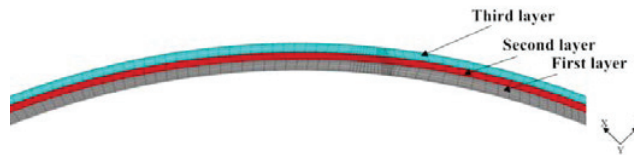
FIGURE 6. Deformed mesh on the outlet surface
