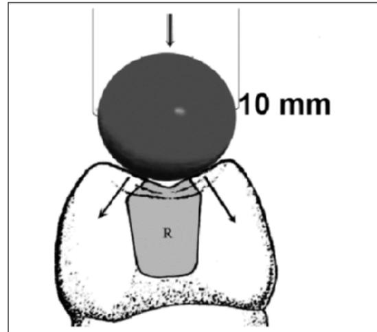
Figure 3: The representation of the load application of the sphere used for the axial compression test.
