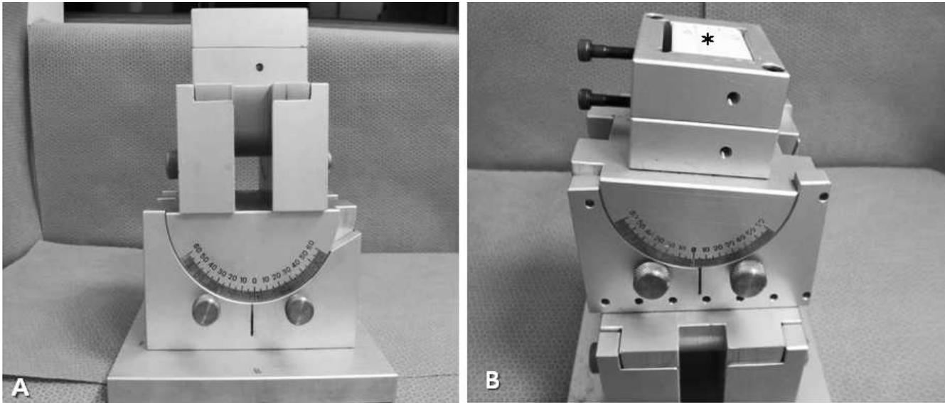
**Figure 6.** (A) Custom-designed and custom-manufactured surveyor system with rotational ability in all three planes. (B) Surgical stent (\*) was placed in the surveyor system. By using the custom-designed surveyor and a CNC machine, a guide hole was drilled in the surgical stent template according to the prescription angles measured on the cone-beam computed tomography data.
