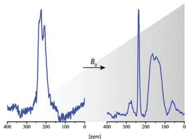
Fig. 5. MAS NMR spectra of  $^{71}\text{Ga}$  in  $\text{Li}_{5.8}\text{Ga}_{0.40}\text{Al}_{0.00}\text{La}_3\text{Zr}_2\text{O}_{12}$  garnet recorded at  $B_0 = 9.4 \text{ T}$  (left) and at  $B_0 = 21.1 \text{ T}$  (right). See text for further details. (Online version in colour)
