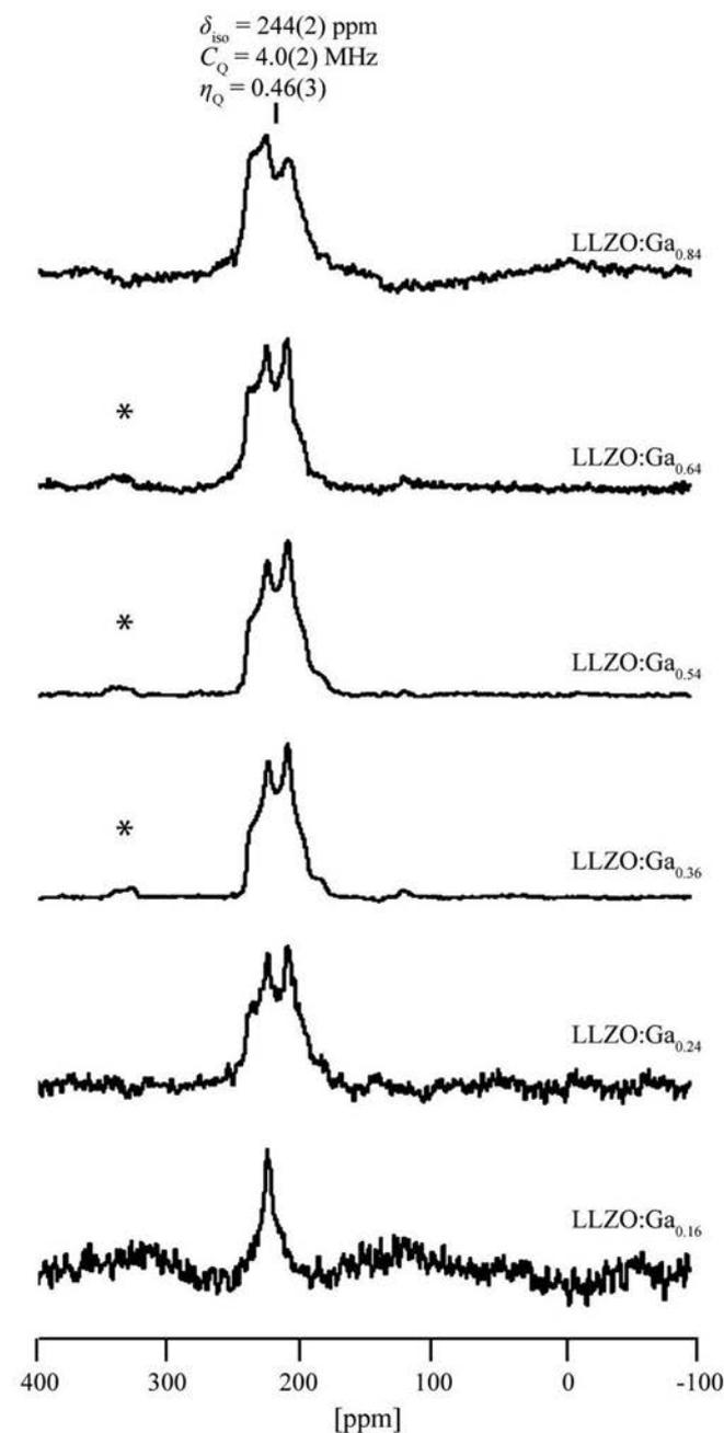
Fig. 7. The <sup>71</sup>Ga NMR spectra of Li<sub>7.3x</sub>Ga<sub>x</sub>La<sub>3</sub>Zr<sub>2</sub>O<sub>12</sub> garnet with 0.16 < *x* < 0.84 taken at 9.4 T (from Rettenwander *et al.* 2014b).
