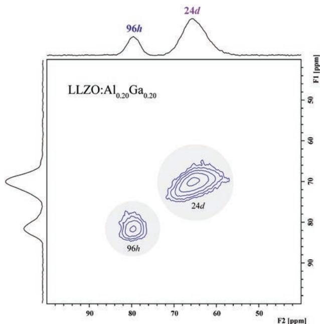
Fig. 6. The 3Q MAS spectra of Ga<sub>0.2</sub>Al<sub>0.2</sub> and Ga<sub>0.0</sub>Al<sub>0.4</sub> recorded at 21.1 T and a spinning speed of 31.25 kHz (taken from Rettenwander *et al.* 2015b). (Online version in colour)
