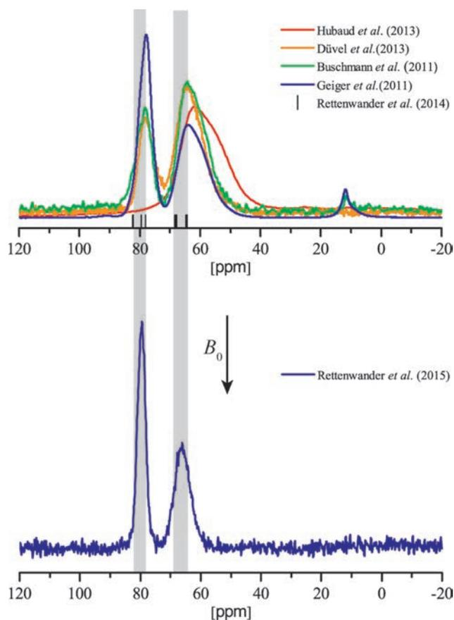
Fig. 4. Top:  $^{27}\text{Al}$  MAS NMR spectra reported from literature measured at low field  $B_0 = 9.4 \text{ T}$ . See text for further details. Bottom:  $^{27}\text{Al}$  MAS NMR spectrum of  $\text{Li}_{5.8}\text{Ga}_{0.00}\text{Al}_{0.40}\text{La}_3\text{Zr}_2\text{O}_{12}$  garnet measured at high field  $B_0 = 21.1 \text{ T}$ . (Online version in colour)
