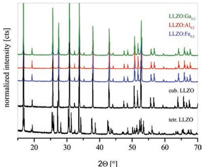
Fig. 2. X-ray powder diffraction pattern of cubic LLZO:Fe<sub>0.16</sub>, LLZO:Al<sub>0.40</sub>, and LLZO:Ga<sub>0.40</sub> (*Ia-3d*), together with the patterns of cubic and tetragonal LLZO from Awaka *et al.* (2009) and Han *et al.* (2012). The XRPD pattern of the whole solid solutions can be found in Rettenwander *et al.* (2013, 2014a and b, 2015a and b). (Online version in colour)
