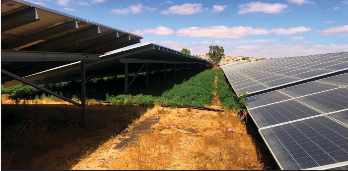
FIGURE 2. Contrast between the untreated soil surface (foreground) and the planted test plot.
