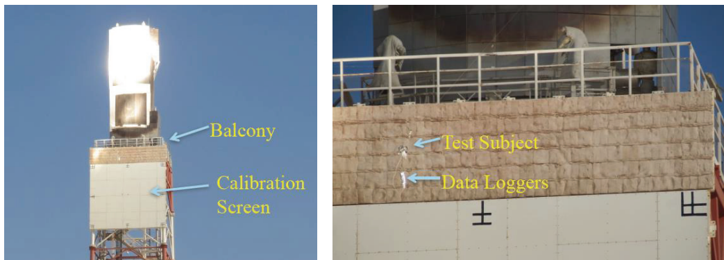
FIGURE 2. Tests conducted by Santolo 7 using bird carcasses exposed to different solar flux levels.
