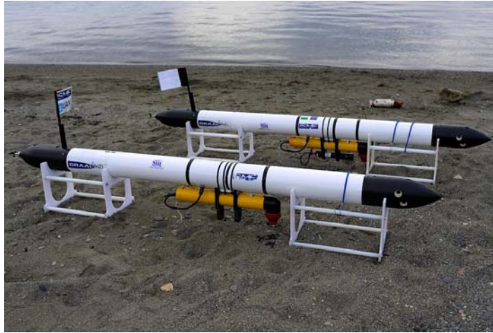
Figure 1: Folagas on shore; the UAN module is visible, mounted at mid-vehicle.
