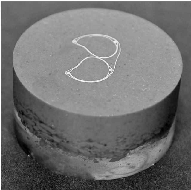
Figure 6. Archwire samples embedded in phenolic resin.
