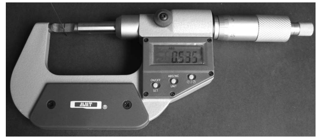
Figure 4. Measuring archwire dimensions using a digital gauge (MMT 0.001 mm, Vogel).
