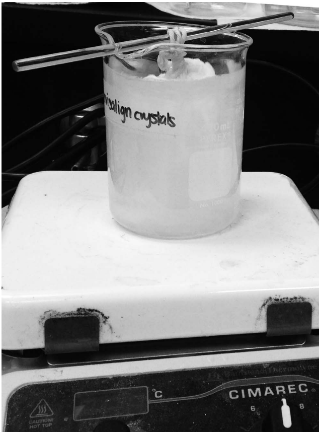
Figure 1. Specimens submerged in a cleaning solution on a magnetic stir plate.
