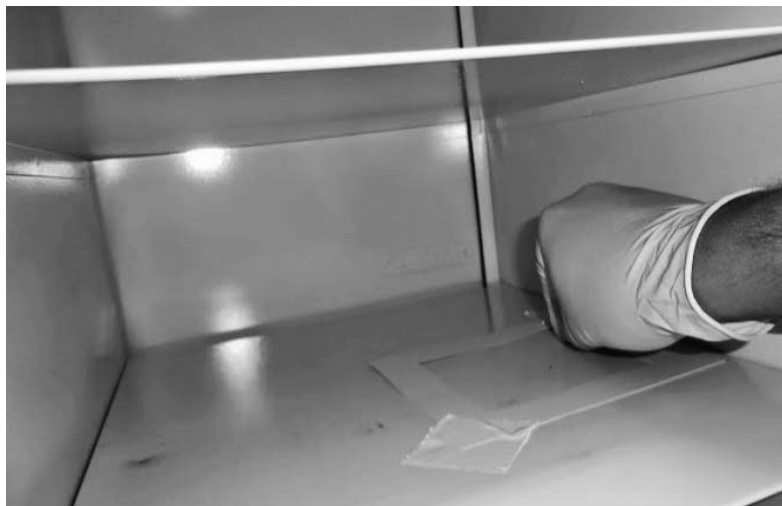
Figure 3. Wipe sampling using Smear Tab and disposable wipe template. Notice the black stains that suggest the presence of mercuric chloride.
