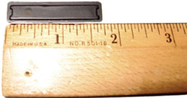
A typical passive RFID tag used with a loss prevention system at a home center store. This tag was removed from a blister pack for cordless drill batteries.
