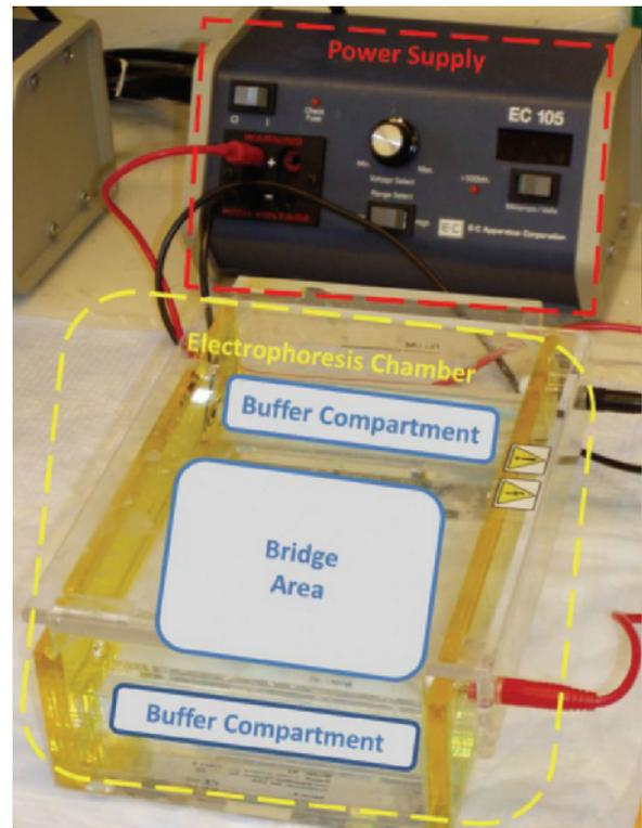
Figure 1. Gel electrophoresis apparatus. Source: [http://commons.wikimedia.org/wiki/File:Gel\\_electrophoresis\\_apparatus.JPG](http://commons.wikimedia.org/wiki/File:Gel_electrophoresis_apparatus.JPG)
