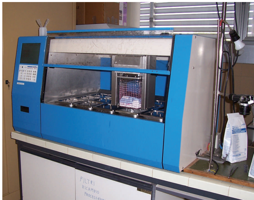
A rectangular moving-basket tissue processor showing the individual containers within the hood.
