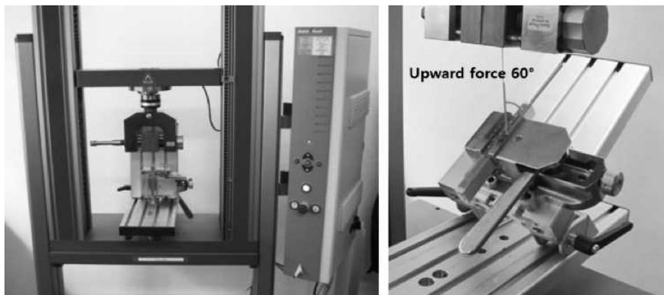
**Figure 2.** Specialized jig system for the application of directional pull-out forces.
