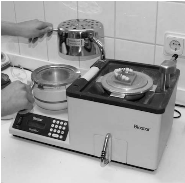
Figure 3. Duplicated model of cold-curing dental resin (Palapress-vario, Heraeus Kulzer, Hanau, Germany) in a Biostar Thermoforming Machine (Scheu Dental).
