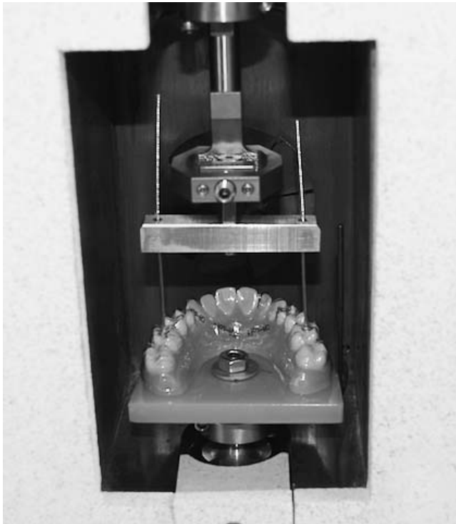
Figure 5. Model inside the GABO Qualimeter Eplexor (GQE). Aligner attached via steel ropes running straight from the first molars through the aligner to the bolting apparatus. The upward displacement force was measured in 10-second intervals until the aligner was removed from the model.
