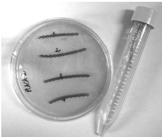
Figure 2. Sample disposition in a Petri dish with agar brain heart infusion and 15-mL test tube with agar brain heart infusion broth.
