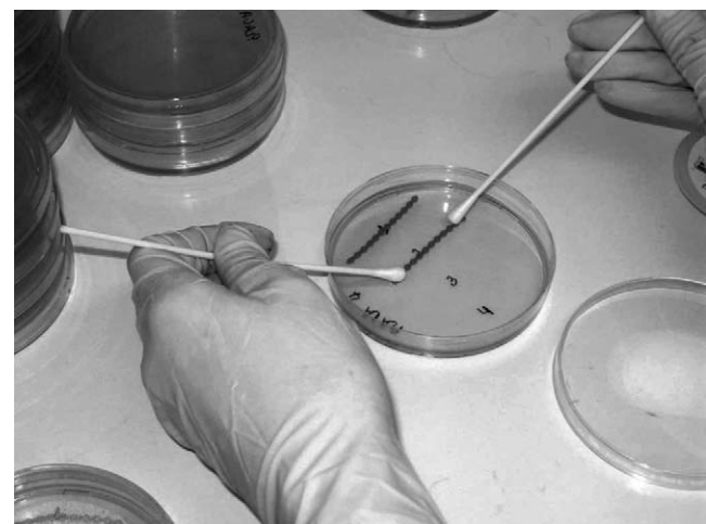
Figure 3. Insertion of the elastomeric chain in the Petri dish with the aid of a swab.
