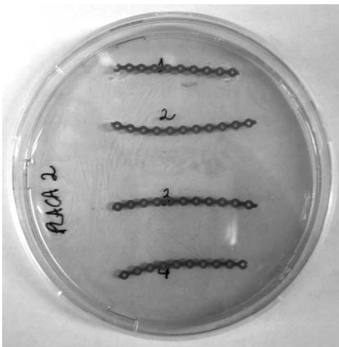
Figure 5. Absence of bacterial and fungal sediments on dish 2 of the elastomeric chain of 3M Unitek. The same pattern without roughness of the elastomeric chain was presented in every sample.
