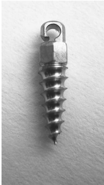
Figure 1. The orthodontic mini-implant used in this study (2005H, ORTHOplant, BioMaterials Korea, Seoul, Korea; self-drilling type, conical shape with 2.0-mm upper diameter, 5-mm length).
