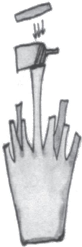
Fig. 9. The flat sides of the larger bell are tapped at the handle end with the Otutu Awka. The bell is thus flattened until its pitch rises to the desired level, whereupon it is left to cool. (© Chiamaka Ezeani)
