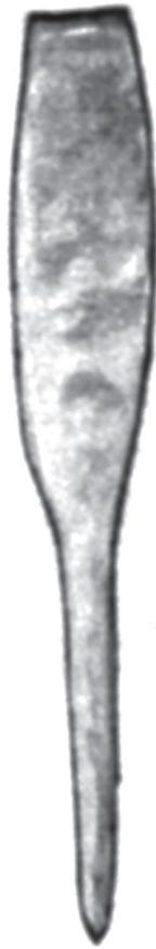
Fig. 1. The Otutu Awka, an iron rod used for beating the hot metal of the bell while it is forged. (© Chiamaka Ezeani)
