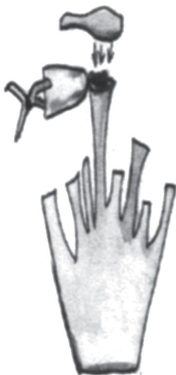
Fig. 6. The Otutu Awka beats the fired end of the bell into a nearly cylindrical form, which is then hammered into a curve. (© Chiamaka Ezeani)
