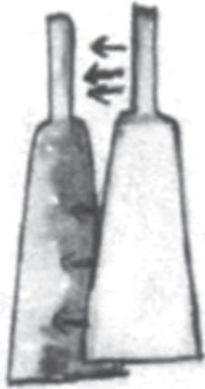
**Fig. 3.** A bell mold is used to trace two identical patterns on a 15–16-gauge metal sheet. The shapes are chiseled from the sheet and bound together with wet earth. (© Chiamaka Ezeani)
