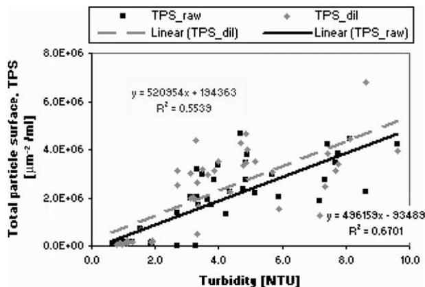
Figure 7 Relation of turbidity and TPS 2–100 µm of raw and diluted measurements
