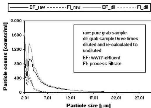
Figure 1 PSD for raw and diluted EF and FI
