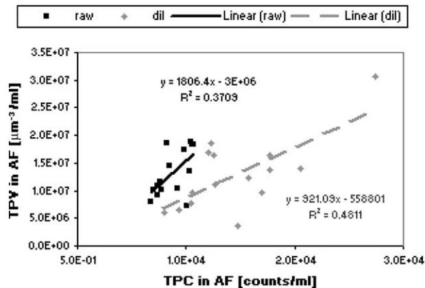
**Figure 4** Correlation between TPC and TPV in AF (2–100 μm) for raw and diluted measurements
