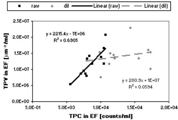
**Figure 3** Correlation between TPC and TPV in EF (2–100 μm) for raw and diluted measurements
