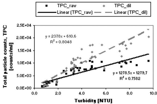
Figure 6 Relation between turbidity and TPC 2–100 µm of raw and diluted measurements
