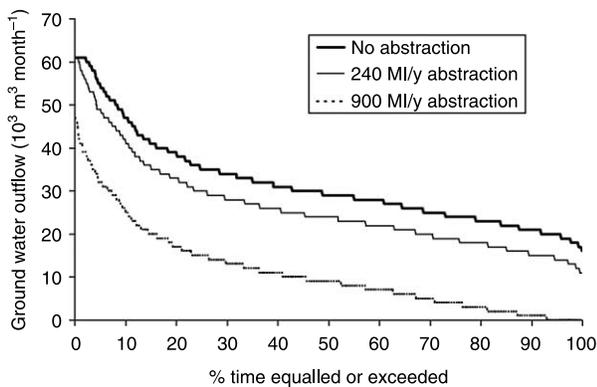
**Figure 4** | Duration curves of simulated (using a rest water level of 25 m) ground water outflow (to a downstream sub-catchment), used as a surrogate for ground water level (within the legend  $MI = 10^3 m^3$ ).
