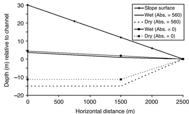
**Figure 5** | Simulated conditions in one slope element of the downstream sub-catchment (213.7 km<sup>2</sup>) with a rest water level parameter value of 15 m and abstraction volumes of 0 and  $560 \times 10^3 \text{ m}^3 \text{ y}^{-1}$  (the slope surface line is arbitrarily positioned).
