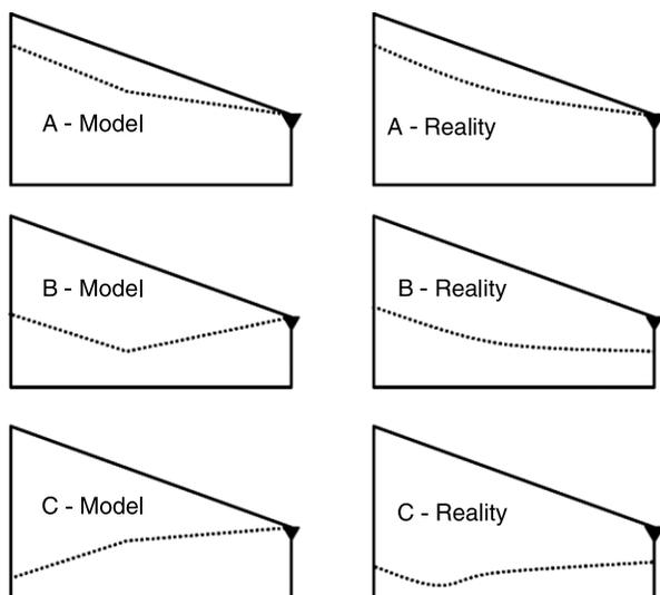
**Figure 2** | Modelled versus real groundwater conditions in a single hillslope element. Dashed lines represent the groundwater levels, the solid upper line represents the surface and the solid triangle represents the river channel. See text for explanation.
